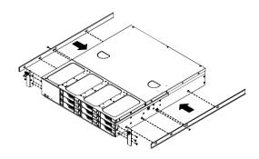
• Mount the outer rail assembly to your rack. Please note that both the front and back of the outer rail assembly will need to be fastened to the rack with two screws.
