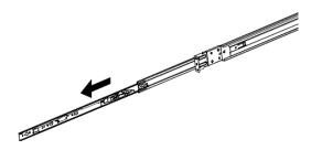
• Press down on the release tab and pull the inner rail out.
