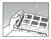
• Slide the disk tray onto the rails of the disk bay. Using the latch, gently push the disk tray all the way into the disk bay. Secure the disk tray in place by pushing down on the latch. The latch should close easily and snap in with an audible 'click'. Please make sure that the disk tray is pushed all the way into the disk bay before attempting to secure the latch.
