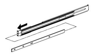
• Line up the holes on the inner rail with the pegs on the system chassis and push the inner rail all the way in.
