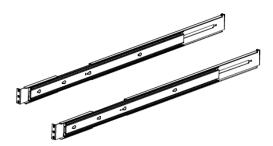
• Fully extend the rail assembly by pulling it outward.
