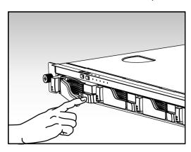
• Using the latch, gently pull the disk tray out of the disk bay.
