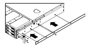
• Mount the inner rails to the system chassis using the provided mounting screws.
