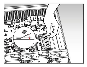
Using two fingers, carefully push down and then back on the memory module until it clicks into place. You should be able to hear an audible "click".
