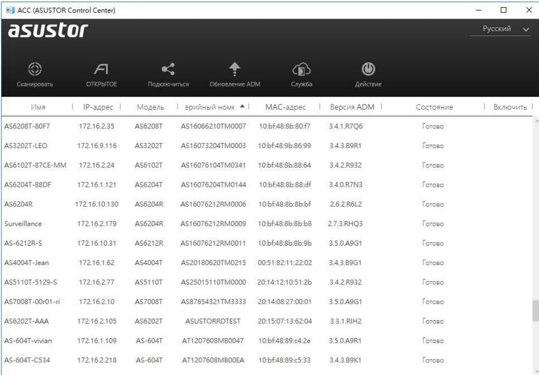
The screenshot shows the ACC (ASUSTOR Control Center) window. The interface is in Russian. At the top, there are navigation icons: Сканировать, ОТКРЫТОЕ, Подключиться, Обновление ADM, Служба, and Действие. Below the icons is a table listing detected NAS devices. The table has columns for Name, IP address, Model, Serial number, MAC address, ADM version, and Status. All devices listed have a status of 'Готово' (Ready).
